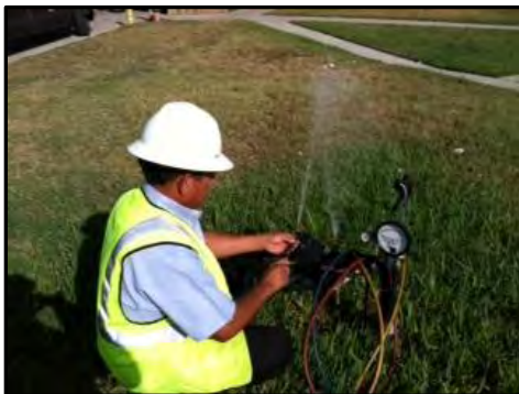
Supervisor Joe Casillas is testing the back flow service line at 509 Wanda Preventer Device at Wastewater Plant
