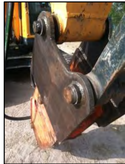
Garage department removes steel on the structure (street department assist) Garage department welds metal plates to attach the hydraulic hammer
