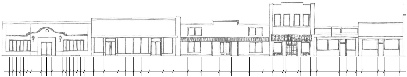
THE GROUND FLOOR RYTHYM IS ESTABLISHED BY THE REPITION OF DISPLAY WINDOWS, DOOR COMPONENTS, AND PIERS WITHIN EACH STRUCTURAL BAY.
