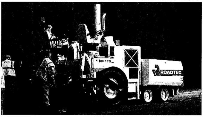
The RP-170 is a rubber-tire asphalt paver with a compact wheelbase for great maneuverability. The RP-170 can achieve a 30" (76cm) turning radius for managing those tight spots around barriers and drains. Fume extraction, adjustable seats, and quiet operation. Quick and easy transportation between job locations.
