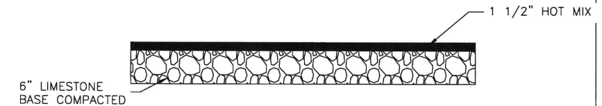
E TYPICAL ASPHALT REPAIR DETAIL 39 SCALE: 1":1'-0"
