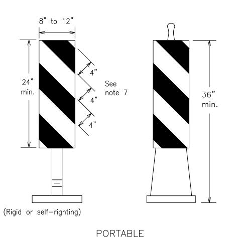
1. Vertical Panels (VP's) are normally used to channelize traffic or divide opposing lanes of traffic.
