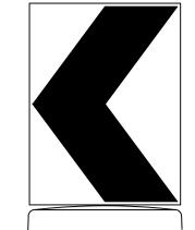
18" x 24" Sign (Maximum Sign Dimension) Chevron CW1-8, Opposing Traffic Lane Divider, Driveway sign D70a, Keep Right R4 series or other signs as approved by Engineer
