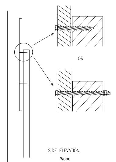
Attachment to wooden supports will be by bolts and nuts or screws. Use TxDOT's or manufacturer's recommended procedures for attaching sign substrates to other types of sign supports
